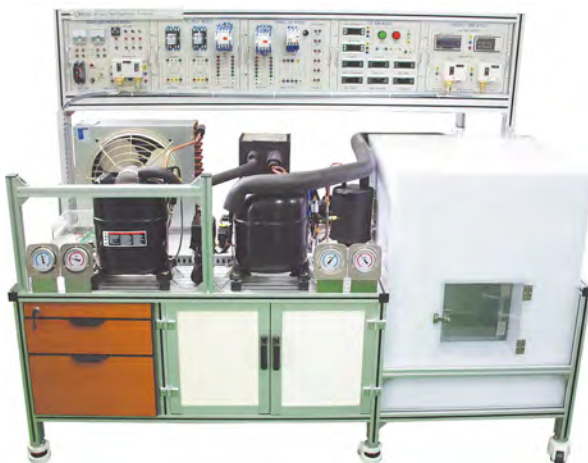
Patent No.0463027 - Binary Refrigeration System Apparatus
