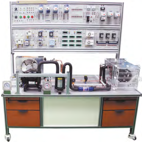
Application Patent No.0293063, Patent No.0473494 - Temperature, Pressure, and Defrost control Refrigeration System Apparatus
