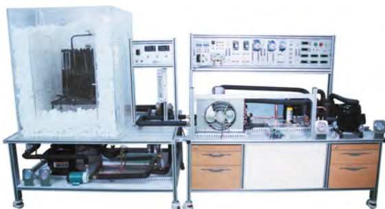
Patent No.0948337 - Heat-Pump System by Geothermal Apparatus
