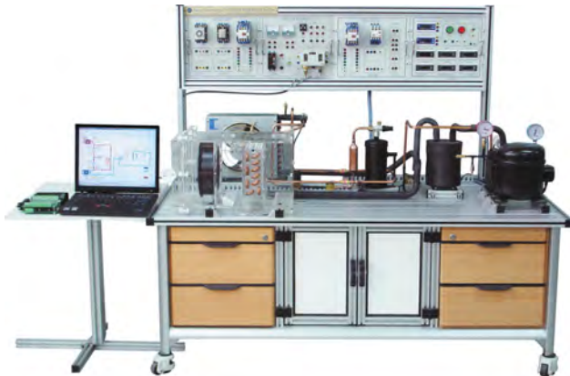
Patent No.0432527 - Heat Pump Heating and Cooling System Apparatus
