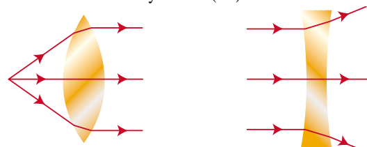
A convex lens gathers the light, and a concave lens spreads the light.
